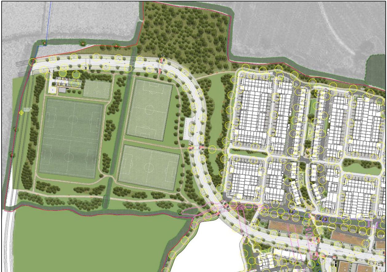
Figure 19 | Proposed Alignment of East-West Link Road through Open Space to Western Boundary
